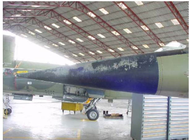
Fig. 8 Alphenet wing leading edge erosion (left) and Mirage F1 nose cone erosion (right)
