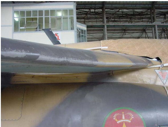
Fig. 8 Alphenet wing leading edge erosion (left) and Mirage F1 nose cone erosion (right)
